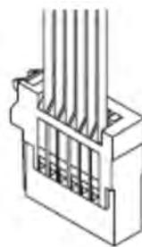
Move the protecting cover in the direction of the arrow to return its original position.
