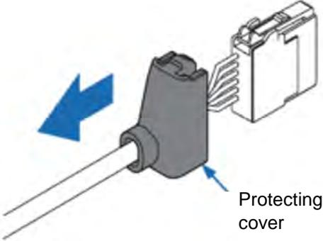
With a flat-blade screwdriver (tip width of 2 mm or less), push in the control lever (white) located at the wire insertion port, and remove the wire.
