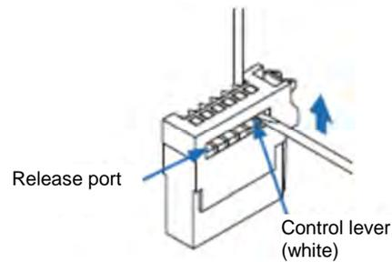
Pull lightly on the wires to check that they are not loose.
