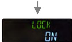
The display will show LOCK ON, and display will then return automatically to the basic screen.
