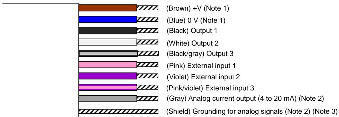
Note 1: Only master units are equipped with +V and 0 V. Power is supplied to slave units through connectors.
