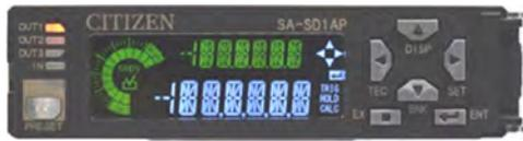
The basic screen appears when the power is turned on.
