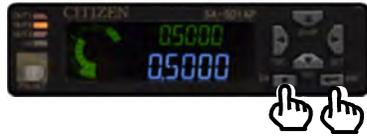
Hold down the ENTER and EXIT keys simultaneously for three seconds.
