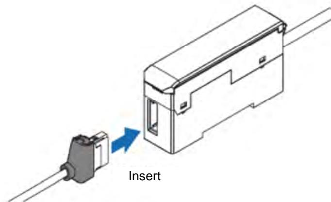
To remove, press the lock release lever on the detector cable controller connector, hold the body of the controller, and—whilst keeping the lever pressed—pull out the connector.
