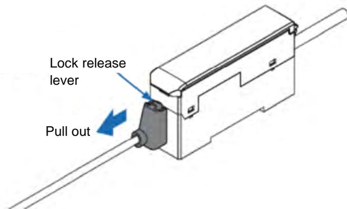
Please note that, when removing the connector, pulling the cable without pressing the lock release lever may result in the cable breaking off or the connector being damaged.
