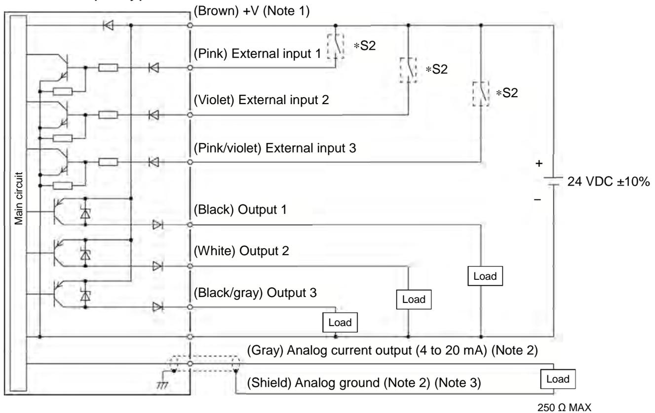
\*S2: Non-voltage contact or PNP open-collector transistor
