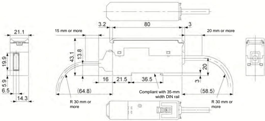
SA-SD1AC, SA-SD1AC-P, SA-SD1C, and SA-SD1C-P
