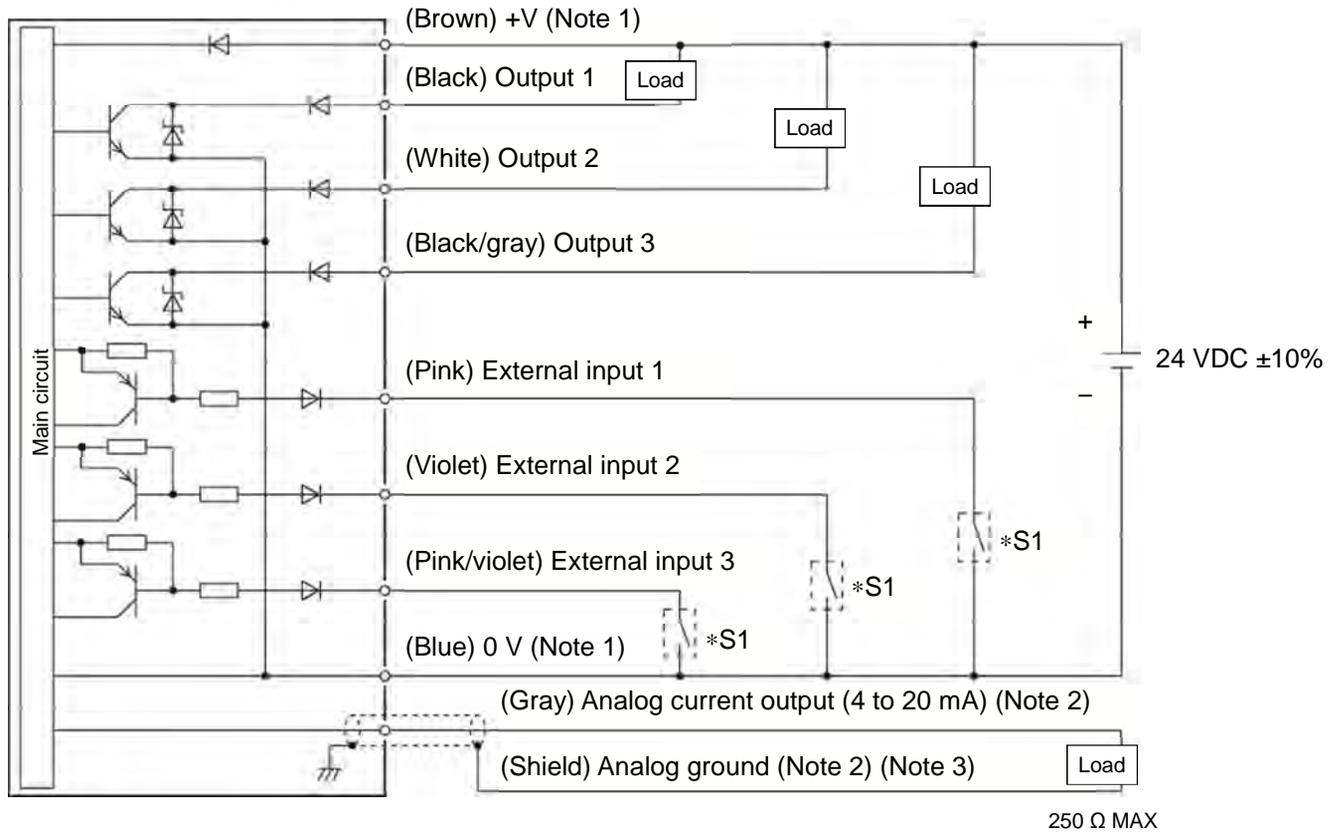
\*S1: Non-voltage contact or NPN open-collector transistor
