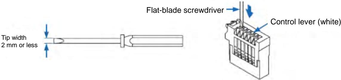
Insert the wire into the wire insertion port as far as it will go. As in the figure below, check that the sheathed section of the wire reaches inside the wire insertion port, and that the tip of the core wires passes through the connection section.
