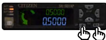
Hold down the ENTER and EXIT keys simultaneously
